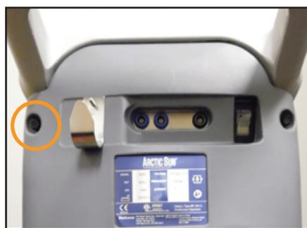
Fig. 8-72 Remova o parafuso (Passo 1)
