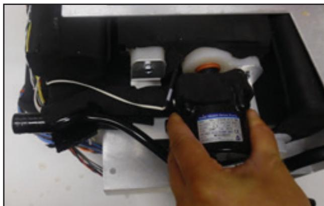
Fig. 8-47 Reinstale a bomba (Passo 6)
